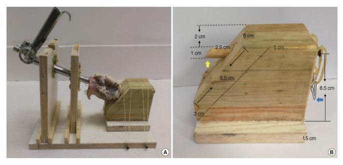
Fig. 1. (A) The simulator with a suspension laryngoscope and the porcine larynx. (B) The porcine larynx can be inserted into the raised portion (yellow arrow) and held by clips (blue arrow). The side length of one component was shown.
