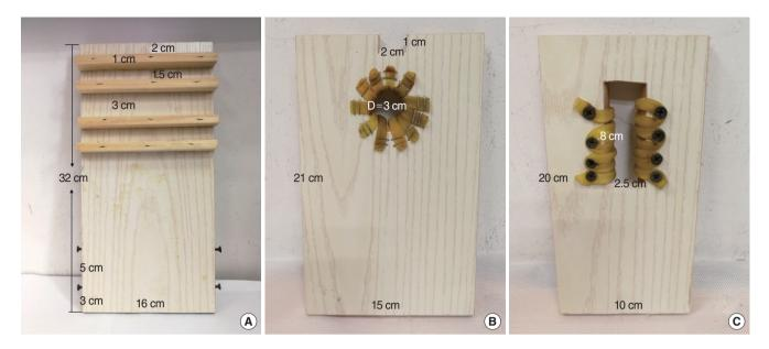
Fig. 2. Three different components of the simulator were made according to the specified parameters. (A) A pedestal with four blocks and four nails. (B) The component to let through the suspension laryngoscope. (C) The component to vertically adjust the suspension laryngoscope. D, diameter.
